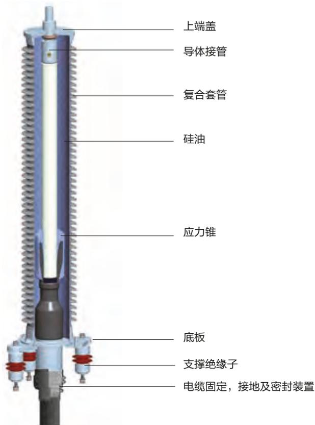
OHVT-245C复合套管户外电缆终端
